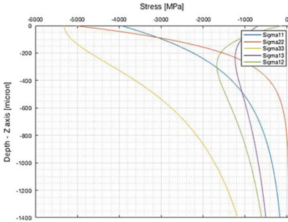
Fig. 41.2 Stress distribution in case of no microinclusions
