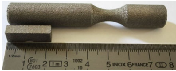
Fig. 14.3 Standard versus miniature as-built fatigue specimens
