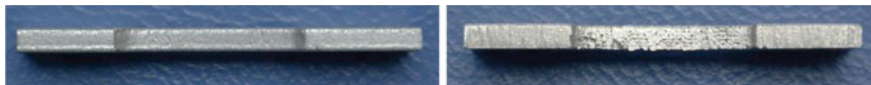
Fig. 15.2 Surfaces of an AlSi10Mg specimen built in the X direction: as-built state (left) and after the removal of support structures (right)
